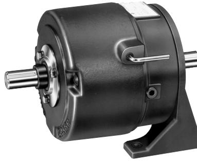
Maximum overhung, or side load measured at one inch from end of shaft: 100 lbs on brake housing side, 150 lbs on endplate/foot mount side
