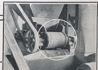
Stearns High Duty Magnetic Pulley Separator removing tramp iron from grain in large distillery.
