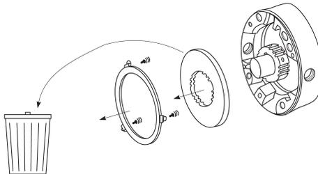
**3** Install new friction disc(s) and stationary disc(s) as shown.
