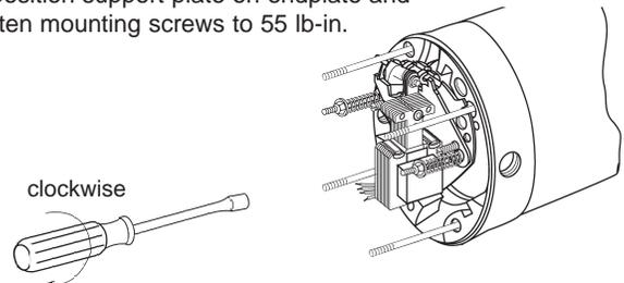
**Note:** Friction discs can wear to 1/2 their original thickness, or .093"
