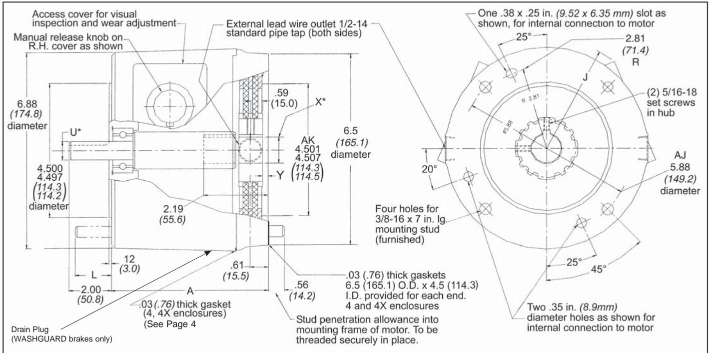
Figure 1 Position hub to Y as shown:
