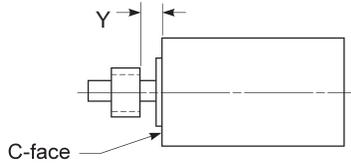
**3** Tighten set screws to motor shaft.
