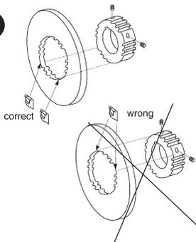
\* Stabilizer clips are for use on single disc units only. Position clips opposite set screw holes.
