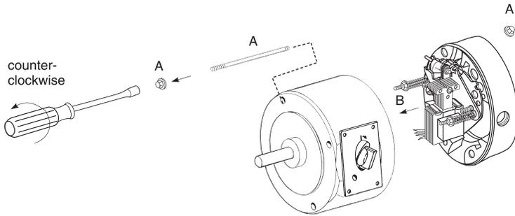
**5** Slide endplate over hub noting position of stabilizer clips, if used. (Refer to Friction Disc Replacement view 3 and 3A). Mount brake endplate to motor C-face using the four tie bolts. Insert minimum 4 turns.
