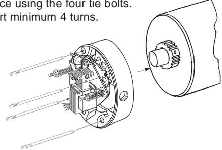
**6** Connect coil lead-wires to power supply. Refer to nameplate for voltage rating.\*
