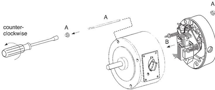
**5** Slide endplate over hub noting position of stabilizer clips, if used. (Refer to Friction Disc Replacement view 3 and 3A). Mount brake endplate to motor C-face using the four tie bolts. Finger tighten.
