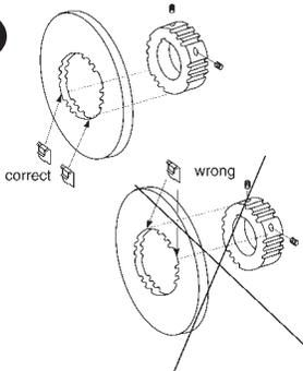
**4** Reposition support plate on endplate and tighten mounting screws to 55 lb-in.
