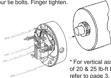
**6** Connect coil lead-wires to power supply. Refer to nameplate for voltage rating.\*
