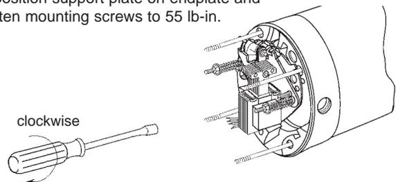
**Note:** Friction discs can wear to 1/2 their original thickness, or .093"
