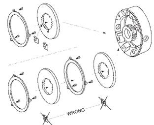
**3A** \* Stabilizer clips are for use on single disc units only. Position clips opposite set screw holes.
