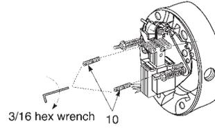
**Note:** Air gap can be adjusted without disassembly. Remove plate (7A) and manual release plate (7B) and adjust as shown above.
