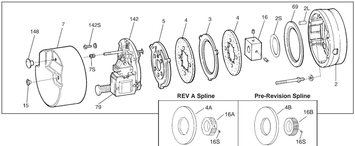
Note color coded sequence of springs and location of washers, if used. Refer to Instruction Sheet 301.3 for proper assembly of vertical mounting components.
