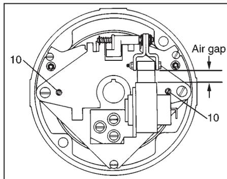
7. The solenoid air gap may be decreased by turning both wear adjustment screws (10) equal amounts clockwise, approximately 1/8 turn, until appropriate solenoid
