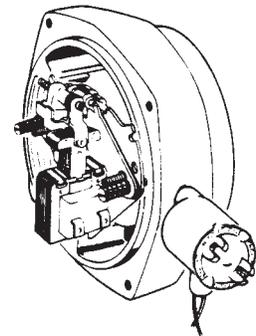
Series 65,300 brakes use four through-bolts (15S) flat washers (15U), lock washers (15W) and hex nuts (15N). Remove all and pull back on housing to free it.
