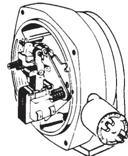
Series 65,000 brakes use four through-bolts (15S) threaded into endplate, and four lock washers (15W). Remove all and pull back on housing to free it.
