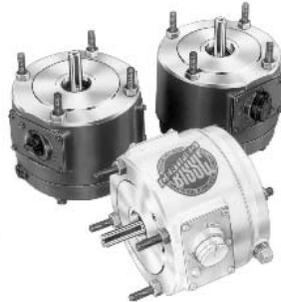
Double C-face brakes are the simple solution for adding a brake to a C-face motor with a single shaft extension. The double C-face allows the brake to directly couple a C-face motor to a C-face gear reducer.
