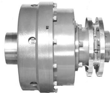
Heavy duty clutches, clutch/couplings, clutch/brakes and brakes for extremely heavy duty high torque applications from 7 lb-ft to 120,000 lb-ft. These rugged units are rotating field, multiple disc friction design and can be custom-built to your application. Consult Stearns Division for your specific design requirements.
