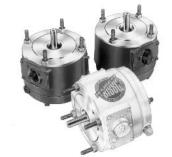
Double C-face brakes are the simple solution for adding a brake to a C-face motor with a single shaft extension. The double C-face allows the brake to directly couple a C-face motor to a C-face gear reducer.
