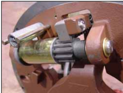
Picture B & C: The correct position of sector gear to pinion with a new disc pack.
