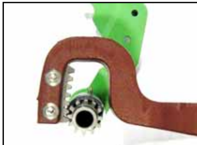
Picture B & C: The correct position of sector gear to pinion with a new disc pack.
